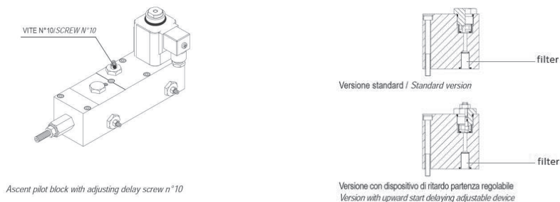
Figure 46 – Filter cleaning of EVS line
